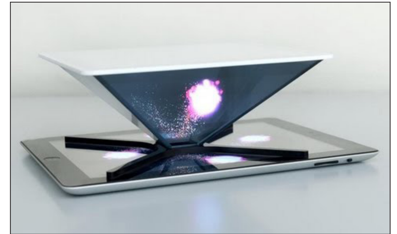
A Holographic Projector used on cellphones serving as a 3d display
